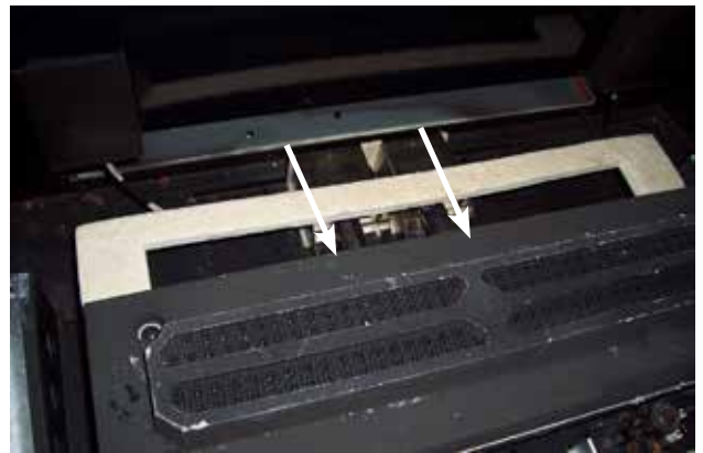
Figure 65: Move Burner away from Mixing Tubes
