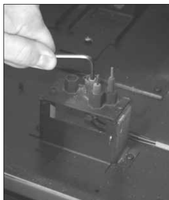
Figure 53: Removing the Pilot Orifice.
