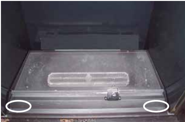
Figure 61: Front Panel Screw Locations
