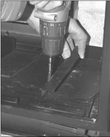
Figure 56: Removing the Right Burner Support.
