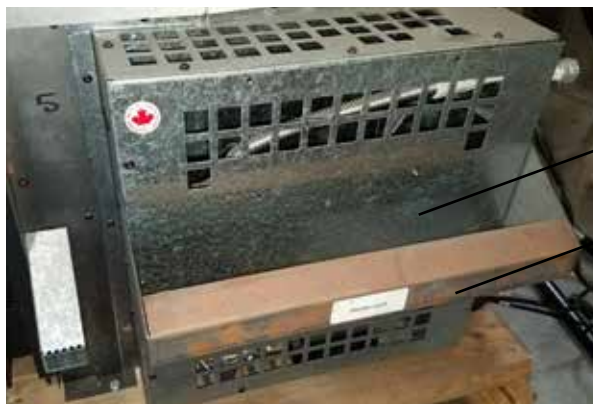
Figure 13: Remove Right Side Handle & Outside Access Door
