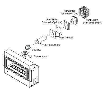
When using Rigid Vent other than Simpson Dura-Vent, 3 screws must be used to secure rigid pipe to adaptor.
