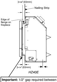
Important: 1/2" gap required between faceplate and finished wall.
