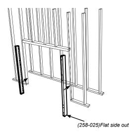
Secure horizontal steel header stud with 2 screws per side as per diagram.
