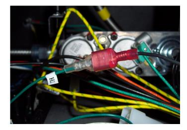
Connect the other thermostat lead to male connector disconnected from Step 1 using a female spade connector - see picture below.
