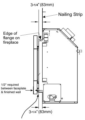
IMPORTANT: 1/2" gap is required between the faceplate and the finished wall when using 4 piece Faceplate (Part # 258-954, 258-957) or Verona Glass Surround (Part # 256-951, 256-957)
