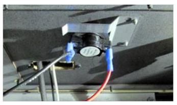
Secure the ground wire from the fan assembly and the power cord to the ground lug located on the back left near the fan.
