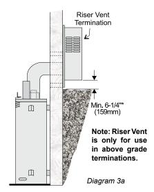
\*Diagrams 3 & 4: As specified in CGA B149 Installation Code. Local codes or regulations may require different clearances.
