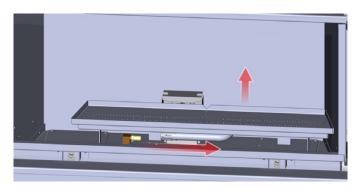
Remove the valve access plate by undoing the 8 screws - see locations below.
