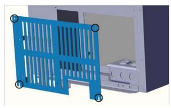
11.Install the fan control module (FCM) into the bracket on the side access panel. Plug in the power cord to the outlet in the unit. Reinstall the panel with the 4 screws from step 10.
