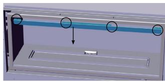
3) Remove installed factory panels. Loosen 2 screws (do not remove) on panel clip securing side panel, Slide panel clip down away from screws. Remove side panel.
