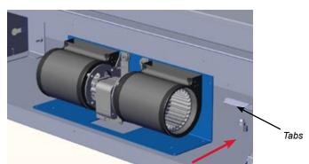
Secure the fan to the floor of the unit with 2 screws, in locations show below.
