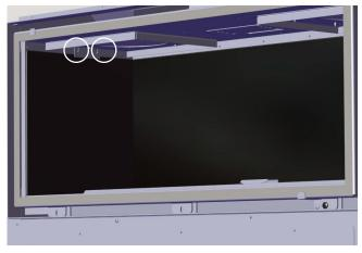
8) Install the right side enamel panel - secure in position with the panel clip and two screws loosened in step 4.
