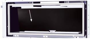
7) Install the left side enamel panel - secure in position with the panel clip and tighten two screws loosened in step 3 as shown in the diagram below.
