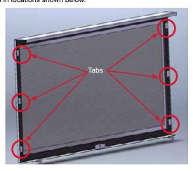
Hook the inner door frame (3) and safety screen assembly (2) over the inner door trim.
