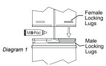
NOTE: For best results and optimum performance with each approved venting system, it is highly recommended to apply "Mill-Pac" sealant (supplied) to every inner pipe connection. Failure to do so may result in drafting or performance issues not covered under warranty.
