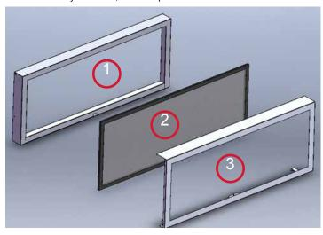
Remove screws from inner side of the inner door trim and discard screws and the brackets. (Brackets not shown). Remove the screen mesh from inner door trim.
