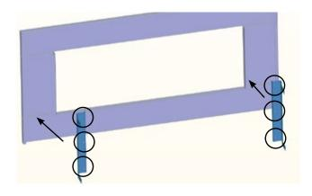
3) To install the 4 piece faceplate - hook brackets (located on back of faceplate) over the two middle tabs on the glass door frame. If thicker finishing materials are used - the faceplate may be adjusted out - up to 1/2".
