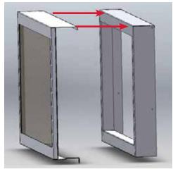
Bend the center tab up and secure with a screw to attach the inner door frame/safety screen assembly to the inner door trim
