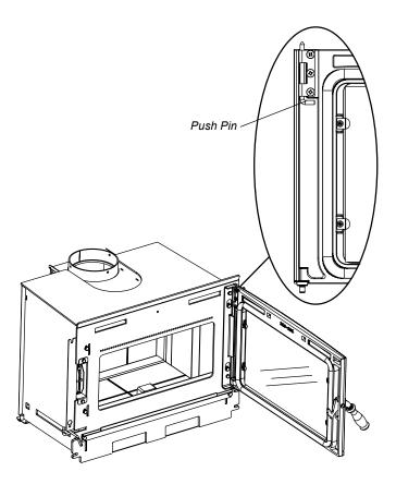
2) NOTE: For Masonry installation make sure that the firebox is level with the hearth using non-combustible materials and no more than 1/2 to 1 inch of the leveling bolt. 3) Lift the unit up onto the Hearth and slide into the fireplace opening. Be sure to leave the unit out at least 3 to 4 inches in order to make the necessary flue connections and to install the fan and faceplate.
