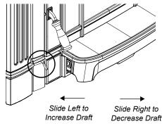
As well as a primary and glass wash air system, the unit has a full secondary draft system that allows air to the induction ports at the top of the firebox, just below the flue baffle.
