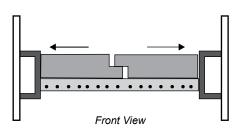
Note: When getting the chimney cleaned, remove the baffle bricks for access to the flue, then replace them when cleaning is completed.
