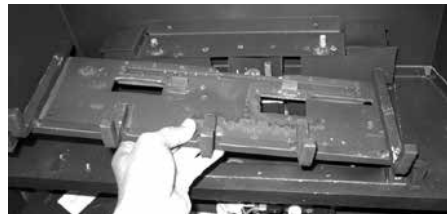
Remove the 2 screws, push Burner Assembly to the left and lift out.
