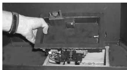
Diagram 1: Remove the left and right screws and then slide the burner/grate assembly to the left and lift out.
