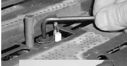
Remove the 2 nuts holding the switch box in place, then pull the thermosdisc out of the bracket.
