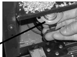
Remove the 2 nuts holding the switch box in place, then pull the thermosdisc out of the bracket.
