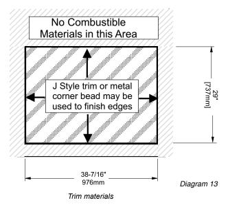
**Note:** All non-combustible facing material should butt up cleanly to the flanges around the firebox opening.
