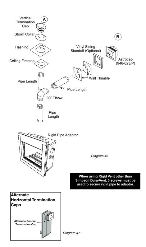
The Regency AstroCap<sup>™</sup> and Regency Riser Vent terminal are certified for installations using Regency venting systems as well as any specific chimney systems listed in this manual. AstroCap<sup>™</sup> is a proprietary trademark of Regency Fireplace Products.
