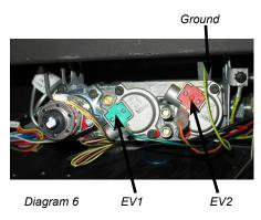
11) Remove the 14 screws securing the valve tray assembly in place (Diagram and then lift the entire assembly out Also remove the valve gasket.
