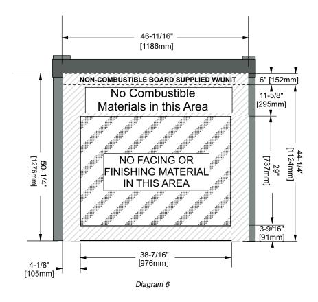
**NOTE:** The 6" x 46-11/16" supplied with the unit is secured directly above the unit as shown above.
