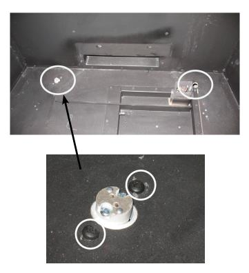
**NOTE:** The ground wire will need to be pulled back out of the protective casing to be able to reach the ground lug. Gently pull the end of the green wire backwards exposing enough wire to reach ground lug.
