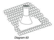
The upper half of the flashing is installed under the roofing material and not nailed down until the chimney is installed. This allows for small adjustments.
