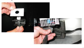
**12)** Install each light assembly from the underside of the floor of the firebox. Secure with 2 screws as shown below.
