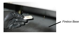
11) Install gaskets onto light assembly mounting plates and feed wires through the underside of the firebox base. Left side shown, repeat for right side.
