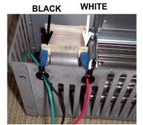
6. Position the fan base with the motor end towards the rear of the firebox and then slide the fan in towards the rear of the unit. Turn the fan housing slightly to the left and make the fan assembly parallel to the rear wall.
