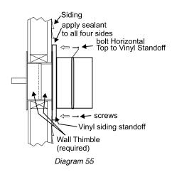
The four wood screws provided should be replaced with appropriate fasteners for stucco, brick, concrete, or other types of sidings.
