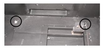
10) Remove the cover plate and gasket from the underside of the floor of the firebox.
