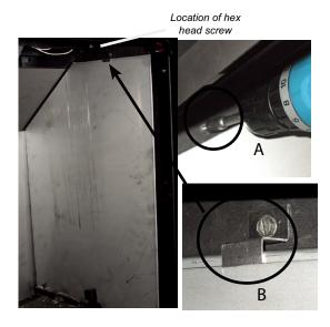
Slide top panel under the top of the back and right side panels as shown below.
