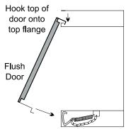
Be careful that the glass gasket does not roll up; there must be a gap between the gasket and the door lip to ensure that the door sits securely on the unit, see Diagram 2.
