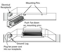
8. Connect and secure fan ground cable to ground lug.
