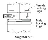
5. Assemble the desired combination of pipe and elbows to the appliance adaptor and twist-lock for a solid connection.
