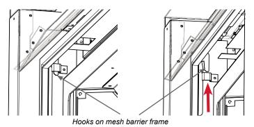
When hooks are clear of the bracket-tilt mesh frame out slightly from the bottom and manoeuvre mesh out.
