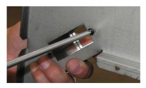
**16)** Reinstall base tray with light diffusers - use caution when installing do not damage the bulb.
