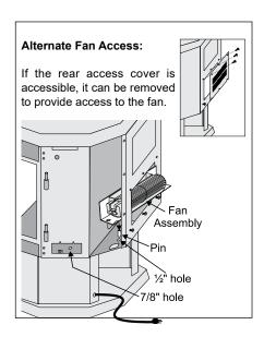
Lift fan off of the 2 pins, tip back and pull through firebox opening. Disconnect the green ground wire from the right side of the fan as soon as you can reach it.
