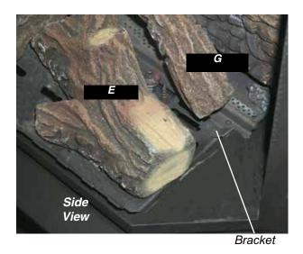
The bottom right edge of Log G must sit snugly against the bracket
