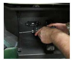
Remove four screws to remove the access panel (in locations shown below) and the chain attached to the front door and the unit.
