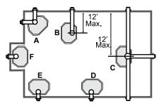
For Vent Termination requirements, see "Exterior Vent termination Locations" section.
