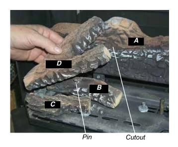
6 Place Front Right Log E on the two pins as shown.
