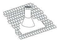
Diagram 11: The upper half of the flashing is installed under the roofing material and not nailed down until the chimney is installed. This allows for small adjustments.
