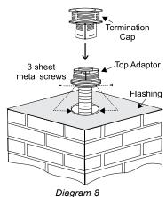
8. Attach the flex to the Retro Connector. Use 3 sheet metal screws to attach the flex liner to the Connector. Diagram 9. Mount the Retro Connector to the masonry wall using masonry bolts. Re-drill larger holes on connector as needed. Be careful to insure that the connector is centered in the opening and the mounting holes line up with the masonry wall.
