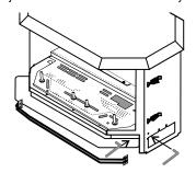
the turning gear which will adjust the air shutter. Open the air shutter for a blue flame or close it for a yellower flame.
