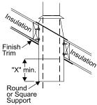
If the support extends above the roof, cut it flush with the top of the roof. Nail the support to the frame opening using (8) 3" spiral nails or #8 x 1-1/2" screws.
