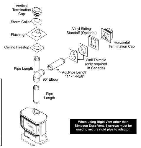
The FPI AstroCap<sup>™</sup> and FPI Riser Vent terminal are certified for installations using FPI venting systems as well as Simpson Dura-Vent® Direct Vent, American Metal Products Ameri Vent Direct Vent, Security Secure Vent®, Selkirk Direct-Temp. AstroCap<sup>™</sup> is a proprietary trademark of FPI Fireplace Products International Ltd. Dura-Vent® and Direct Vent are registered and/or proprietary trademarks of Simpson Dura-Vent Co. Inc.
