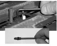
**12.** Remove burner orifice with a 1/2" wrench while using a 9/16" wrench to hold onto the elbow behind the orifice, then discard the orifice.
