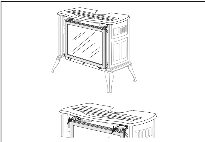
Figure 89 - Release the latches to remove the glass frame.
