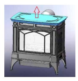
2) Unscrew upper rear panel mounting screws using Phillips head screw driver.
