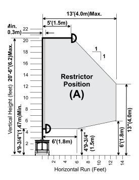
NOTE: See "Vent Restrictor Position" section for installation instructions for the Vent Restrictor Position.
