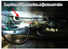
Pull adjustment wire up to close or down to open aeration.
