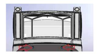
Slide the casting out of the base plate and the side bracket key hole slots and lift the front casting off the unit.
