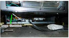
Run the fan grey wire through the small grommet power cord from the valve cover plate to the base panel through the large grommet.
