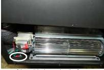
Open the bottom cover of the unit by loosening the 2 screws and removing one from the left side of the unit (when facing back of the unit).
