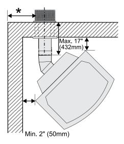
\*If this is an outside corner, the minimum distance between the vent and the outside corner is 6" (15cm). See "F" on the diagram in the "Exterior Vent Terminal Locations" section.
