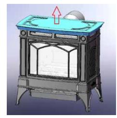
2) Undo the top cast grill mounting bolts using 7/16" or 11mm socket.
