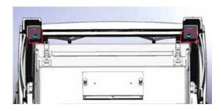
6) Open the valve access door and loossen the bottom front casting bolts using the same tool.
