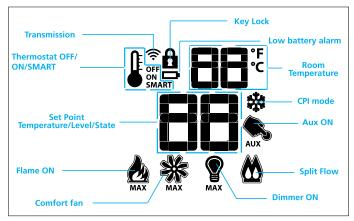
Figure 2: Transmitter LCD Display
