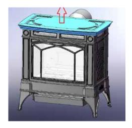
Remove top cast grill mounting bolts using 7/16" or 11mm socket.
