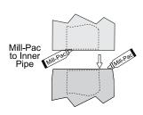
NOTE: For best results and optimum performance with each approved venting system, it is highly recommended to apply "Mill-Pac" sealant (supplied) to every inner pipe connection. Failure to do so may result in drafting or performance issues not covered under warranty.
