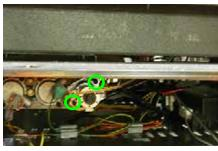
Remove NG Stepper motor and replace with LP Stepper motor
