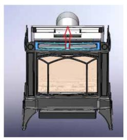
6. Slide safety screen upwards to remove.
