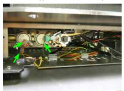
15) Remove two (2) ignition cables from the IFC.
